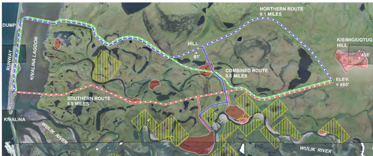
Figure 23: Detail of evacuation routes studied by WHPacific in 2014. The concept project follows the southern alignment over the lagoon shown in red.
